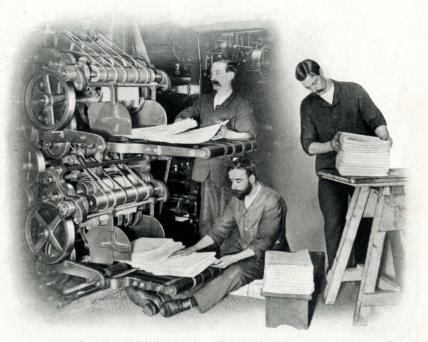
Printing machine delivery mechanism.
